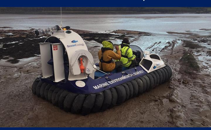
The MACV 'Sepiola' is a twin engine purpose-designed, ultralight Coastal-Pro hovercraft, providing a high specification, multi-use survey platform for a variety of intertidal and coastal requirements.
