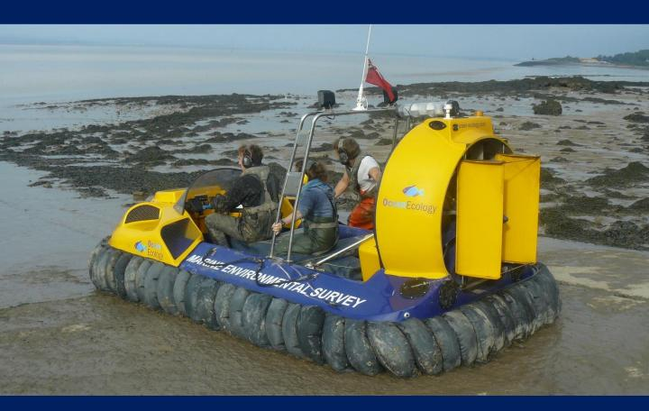
The MACV 'Solea' is a twin engine purpose-designed, ultralight Coastal-Pro hovercraft, providing a high specification, multi-use survey platform for a variety of intertidal and coastal requirements.
